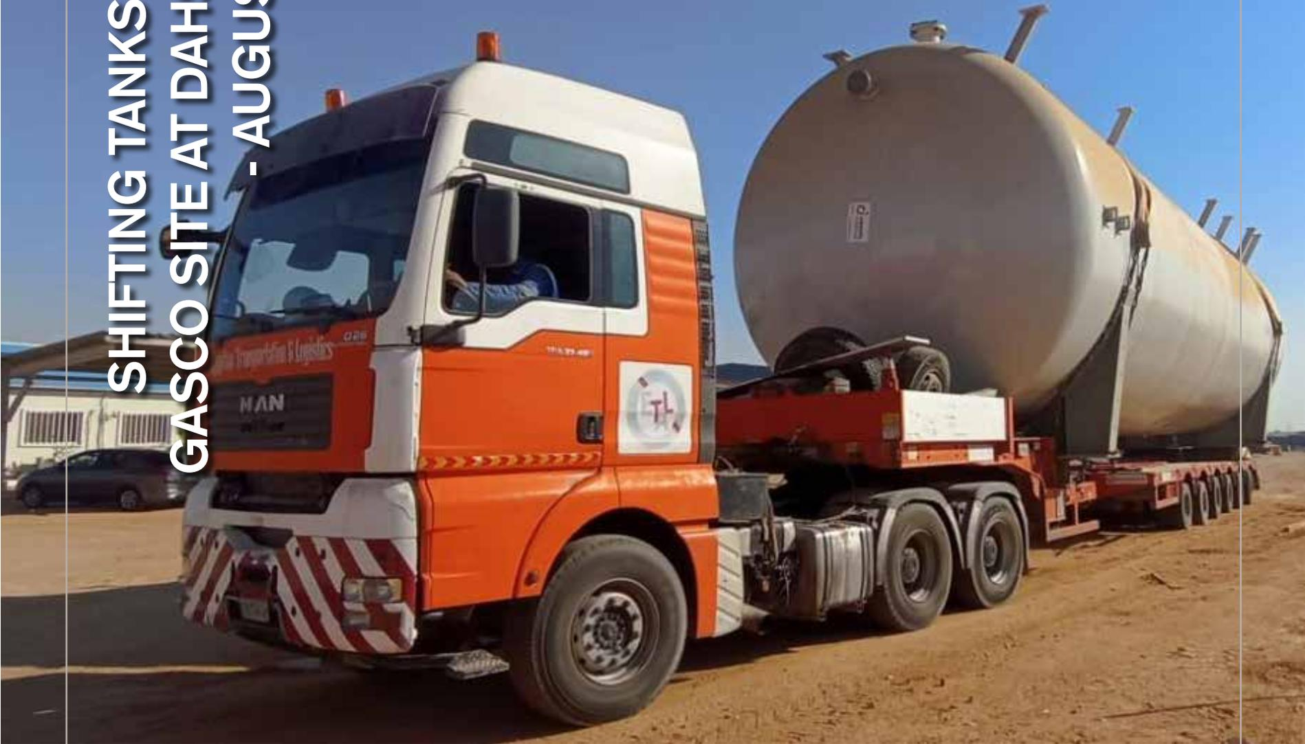
Shifting 6 Tanks(15\*3.20\*3.9) inside GASCO site at Dahshour using a Superflex trailer. (NOSCO)
