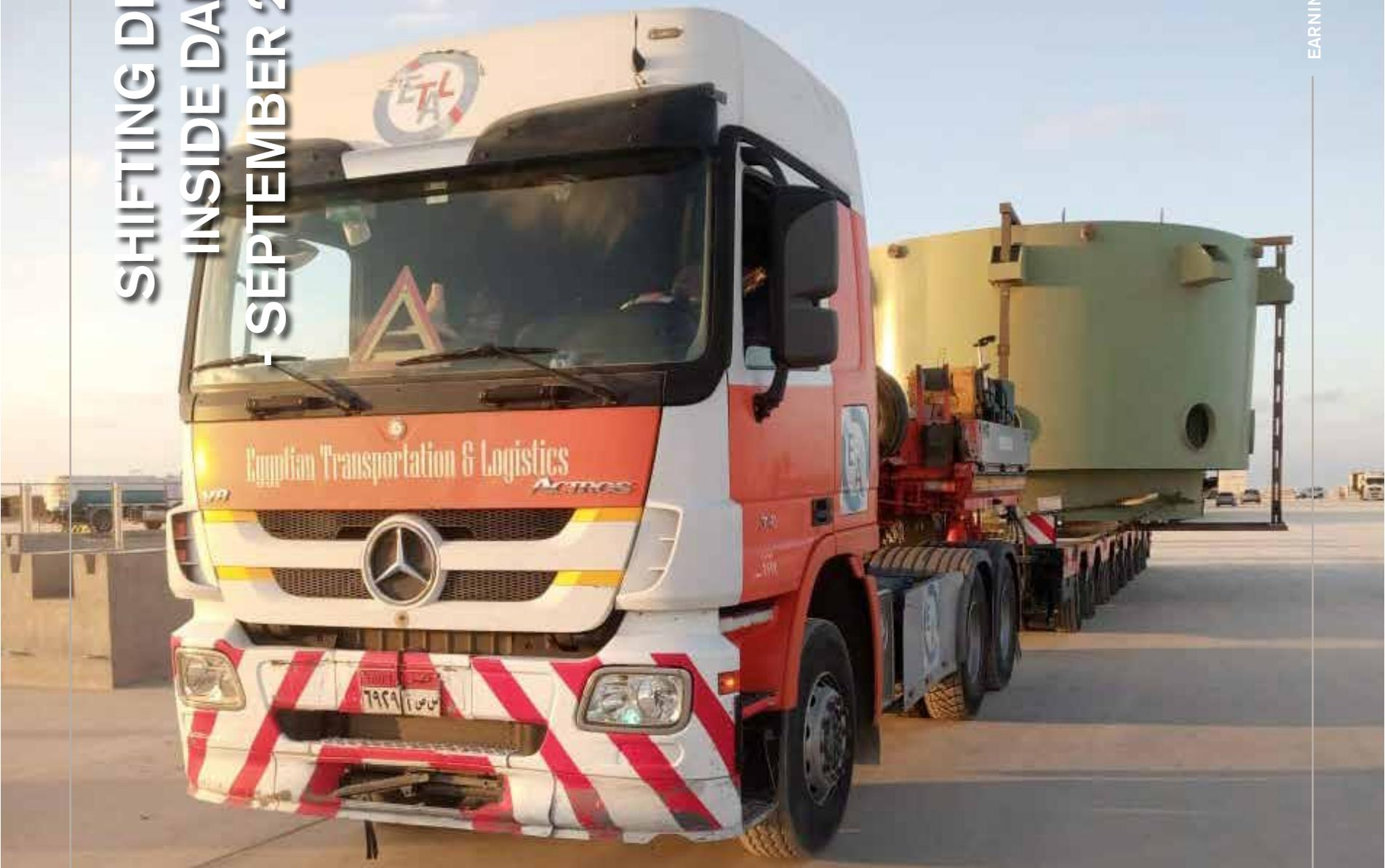
Shifting 1 Drum (7.10\*7.10\*4.15) inside Dabaa port using Superflex trailer.
